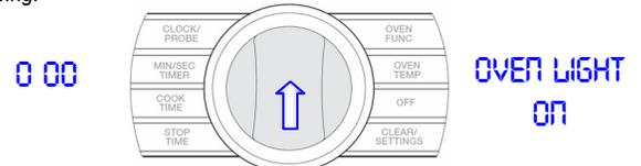
The right display shows that the **Oven light** has been energized. The number in the left display shows the amperage draw on that particular element. The light inside the oven cavity will illuminate
