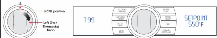
As you advance from 200°F-500°F the SETPOINT reading should coincide with the dial on the knob ( $\pm 5\%$ ). The left display should also vary between 116 (200°F) and 684 (500°F). This will test the thermostat potentiometer.
