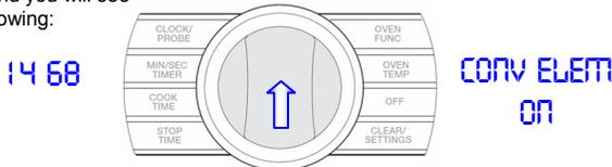
The right display shows that the **Inner Broil element** has been energized. The number in the left display shows the amperage draw on that particular element. Depending on the voltage, the reading can vary. The element will remain on for 1 minute then shut off.
