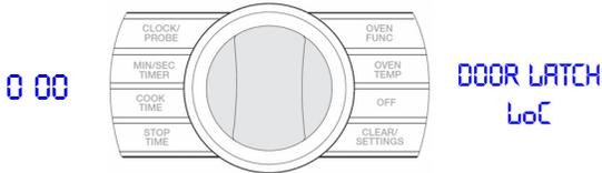
To open the door, simply press in the selector knob and the process will start to open the door.
