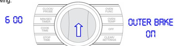
The right display shows that the **Outer Bake element** has been energized. The number in the left display shows the amperage draw on that particular element. Depending on the voltage, the reading can vary. The element will remain on for 1 minute then shut off.
