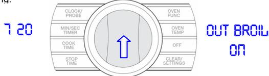
The right display shows that the **Outer Broil element** has been energized. The number in the left display shows the amperage draw on that particular element. Depending on the voltage, the reading can vary. The element will remain on for 1 minute then shut off.
