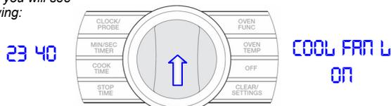
The display shows **Cooling Fan Speed L** and the fan motor has been activated and will run for 1 minute.
