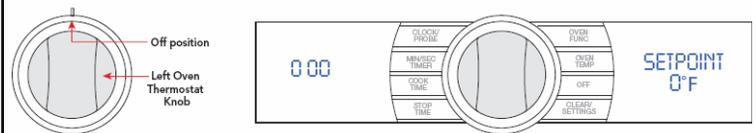
Rotate the **Thermostat Knob** clockwise to the **CLEAN** function. In the left display will be the approximate resistance reading of the thermostat potentiometer (readings may vary by  $\pm 10\%$ ). The right display shows **820°F**.
