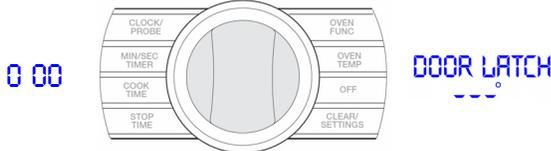
Once the door has locked, the display will change and show the door has locked
