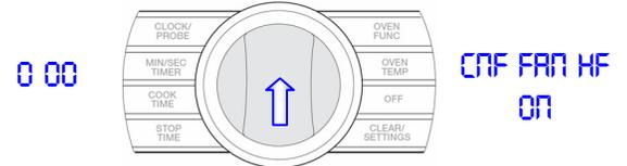
The display shows that the **Convection Fan High Forward** has been activated. The number in the left display shows the amperage draw on the fan motor. The convection motor will run High speed in a clockwise rotation for 1 minute.
