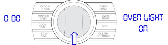
The right display shows that the Heat Light has been energized. On the VDSC548T, the left heat light will be activated.
