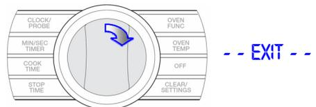
Depress the CLEAR/SETTINGS button to return to main EOC test screen or OFF to exit the diagnostics testing
