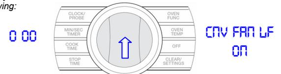
The display shows that the **Convection Fan High Reverse** has been activated. The number in the left display shows the amperage draw on the fan motor. The convection motor will run High speed in a Counterclockwise rotation for 1 minute
