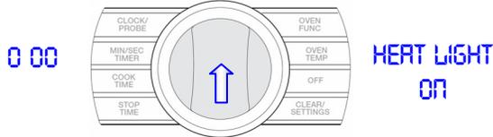
The right display shows that the Heat Light has been energized. On the VDSC548T, the left heat light will be activated.
