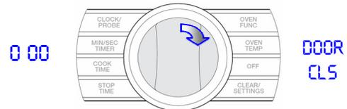
Now, open the oven door. The oven cavity light should illuminate, and the right display will change to show: **DOOR OP n**
