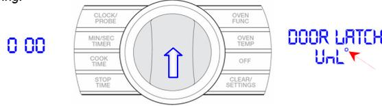
The first thing you will see is that the temperature symbol under the "L" in Latch has illuminated. This indicates that the door motor has been activated. The motor will begin to turn and lock the door.
