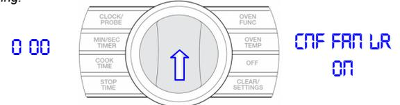
The display shows that the **Convection Fan High Reverse** has been activated. The number in the left display shows the amperage draw on the fan motor. The convection motor will run Low speed in a Counterclockwise rotation for 1 minute.
