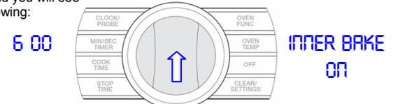
The right display shows that the **Inner Bake element** has been energized. The number in the left display shows the amperage draw on that particular element. Depending on the voltage, the reading can vary. The element will remain on for 1 minute then shut off.
