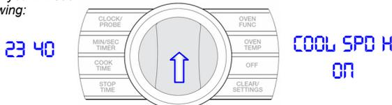
The display shows **Cooling Fan Speed H** and the fan motor has been activated and will run for 1 minute. The number in the left display shows the RPM's of the fan motor as monitored by the Hall Effect Sensor.
