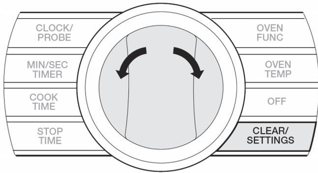
On the VDSC530, 36 and 48T series, to access the programs, push and hold **CLEAR/SETTINGS** button for 3 seconds to access *Settings*.
