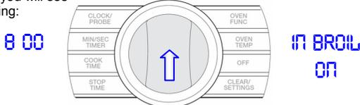
The right display shows that the **Inner Broil element** has been energized. The number in the left display shows the amperage draw on that particular element. Depending on the voltage, the reading can vary. The element will remain on for 1 minute then shut off.
