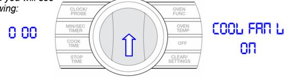
The display shows that the **Cooling Fan Low** has been activated. Amperage shown in the left display. The fan will operate
