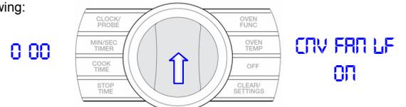
The display shows that the **Convection Fan Low Forward** has been activated. The number in the left display shows the amperage draw on the fan motor. The convection motor will run Low speed in a clockwise rotation for 1 minute.
