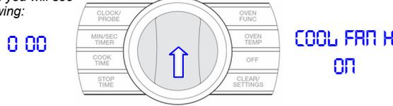
The display shows that the **Cooling Fan High** has been activated. Amperage shown in the left display. The fan will operate
