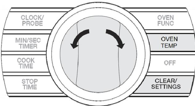
From any of the Settings parameters, press and hold simultaneously the **OVEN TEMP** and **CLEAR/SETTINGS** buttons for 5 seconds and the right display will show: **OFFSET 0°F**
