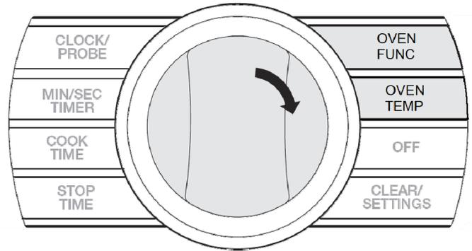
With -- EXIT -- in the right display, turn and hold the Selector knob > Clockwise until a single beep is heard. Release the selector knob. Now, within 3 seconds, press **OVEN FUNC**, then **OVEN TEMP**, then **OVEN FUNC**. If successful, you see the interface software version in the right display **VERSION 16** (16 is the current software version).
